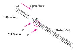
2 Secure L Bracket to outer rail with 1 or 2 M4 screws. Do not tighten yet.
